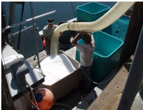
Photo: Ice pumped into the hold of a hook and line vessel, Morro Bay Municipal Dock.
